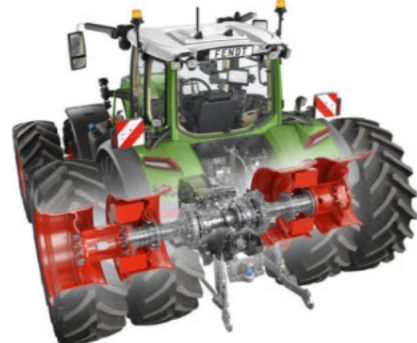
Stub rear axle 3,000 mm twin tyres with dual wheel hub
